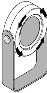
Turn the outer ring on the lampshade anticlockwise as far as it will go to unlock the lampshade.
