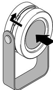
Push the lampshade in as far as it will go and turn the outer ring clockwise as far as it will go to lock the lampshade.
